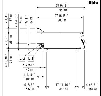
EI = Electrical inlet (power) **EQ** = Equipotential screw
