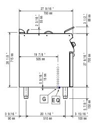
EQ = Equipotential screwG = Gas connection
